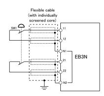
Note4. ISO 13849-1 category and PL need to be evaluated on the entire safety system Note5. The contactors K1, K2 must provide mirror contacts in accordance with IEC 60947-4-1
