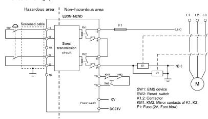
Note. Any possibility of a short-circuit between the conductors connected to the output terminals 13 and 24 must be excluded by constructive measures in the equipment design.
